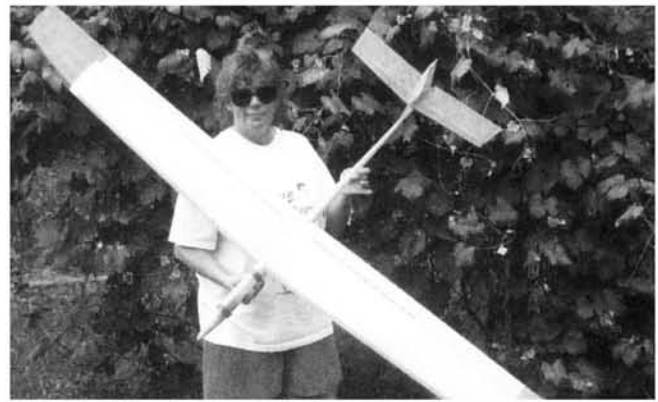
heavy (56 ounces) 2-meter Duck (above left) and the much lighter (23 ounces) 2-meter Dove II (above right). That's his lovely wife Sue holding both planes.
